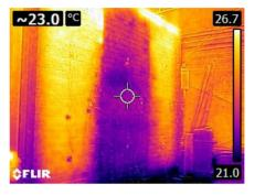
Bricks coated with ProPERLA were found to be more energy efficient than uncoated ones. The thermal image here was taken of the rear of the wall during a rain cycle and it clearly shows a 6°C temperature differential between coated and uncoated bricks. The uncoated brick panel is in the middle.
